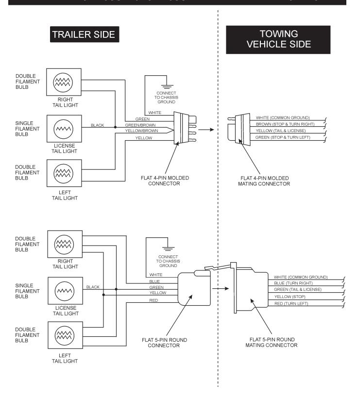
Figure 58. Trailer/Towing Vehicle Wiring Diagram
